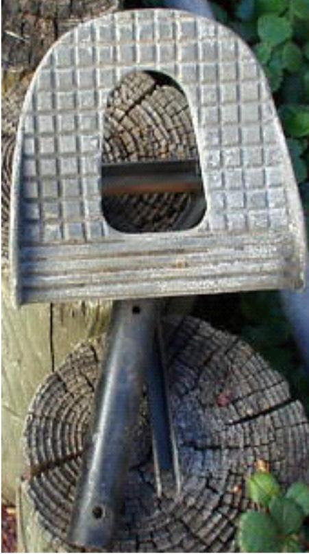
The pilot's side of the cast rudder pedal from a '46. This is an original, with no paint. Note the lack of any wear...this from the right side.
