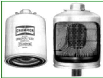
It is critical to understand the difference in the filters since they all look the same, but differ as to the internal features as well as the "gender" of their attachments. On the far left, the "female" 48108-1 model which is the one meant to be used with the F&M filter adapter. On the right, the "male" 48110 filter, showing that it comes with the threaded fitting. Its image is larger to show more detail but they are actually the same
