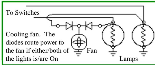
One of the suggestions to keep the lamps cool in continuous use is to add a fan so picture a small computer fan mounted on the rib within the lightening hole in the picture. Four ounces perhaps, made for thousands of hours of run, 12 Volts, 70 milliamps (0.070 A), and 2-1/2 inches square and an inch deep.
