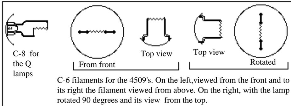
Note that if the Q lamp is rotated by 90°, the filament orientation would still be horizontal, front to rear. For the 4509, some rotate them 90° to have the filament vertical, trying to get greater vibration resistance of the filament when vertical versus when horizontal and accepting the penalty of the loss of beamwidth.
