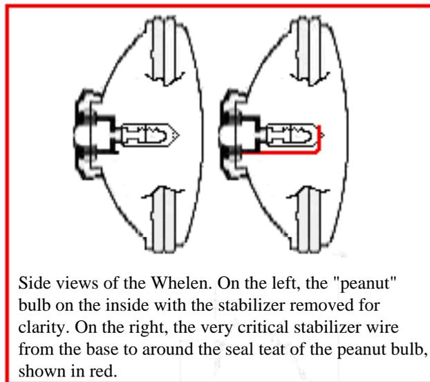
Side views of the Whelen. On the left, the “peanut” bulb on the inside with the stabilizer removed for clarity. On the right, the very critical stabilizer wire from the base to around the seal of the peanut bulb, shown in red.
