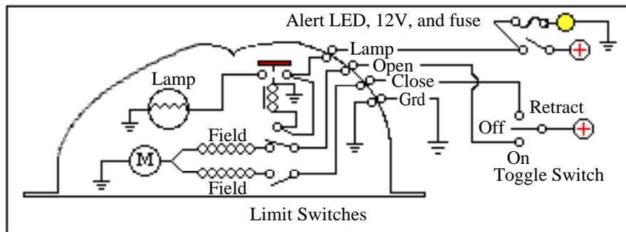
The simplest change; connect a wire between the input power terminal and the relay coil as shown. When the new switch in the Lamp circuit is closed, the relay closes and the power is applied to the lamp, whatever the position of the light itself. And the alert light recommended to prevent forgetting that the lamp is on is also shown wired from the new switch in the Lamp circuit. The extra fuse for it is to do what fuses do; protect the wire to the LED.
