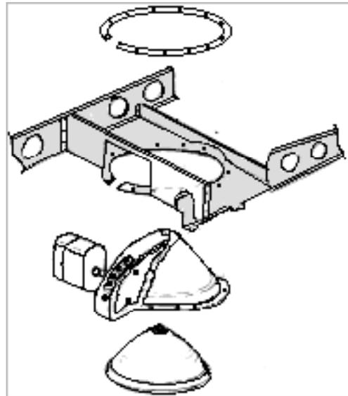
Figure 62/pp119 of the Cessna 120/140 Parts Catalog shows the best representation of the landing light, bracket, fuses, and switches but realize that many of the light assemblies did not look exactly as shown. Note on the parts callout for that figure that some planes had both left and right light brackets as part of the wing assemblies and some did not. The kits were set up to accommodate planes with one or both brackets. The kits included the fuses, holders, light assemblies, and switches.
