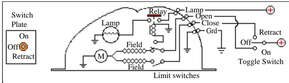
You can arrest the downward or upward motion by flipping the switch to Off and you can move the switch to Retract before the unit is all the way down, or to Down before it is all the way up, but nothing will happen and you must let the initial movement complete and the limit switch reverse before you can change direction. You can stop the movement anywhere you want, but the lamp only lights when full down in the “normal” lights.
