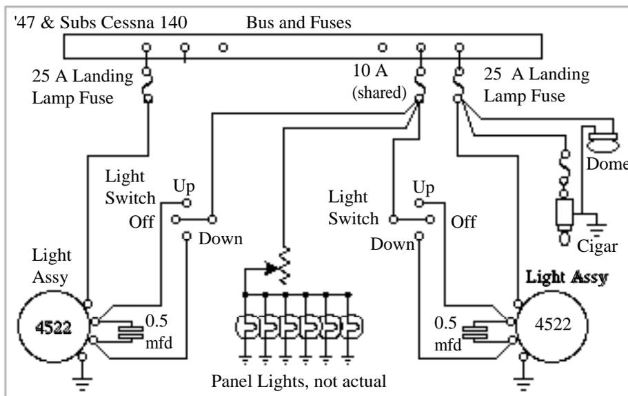
Another change was to let the common 10 A fuse supply the panel lights and both Retract/Down switches. By this time, Cessna had changed to six panel lights with a rheostat for dimming. The panel light rheostat is indicated without an off position because that is how Cessna shows it but actually had an Off position.
