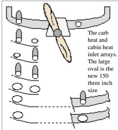
The carb heat and cabin heat inlet arrays. The large oval is the new 150 three inch size
