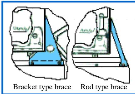
150 exhaust pipe extensions require a stabilizer secured to an oil tank stud
