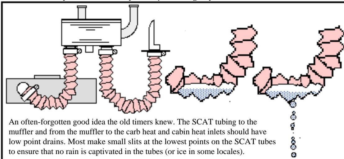
Making these slits takes intestinal fortitude the first time but we are all believers because our timing to do it was after a wash, a careful wash, and the amount of water that came out of the tubes was....surprising. With the slits, you will never ingest a slug of water in the engine, and you won't get sprayed in the cabin
