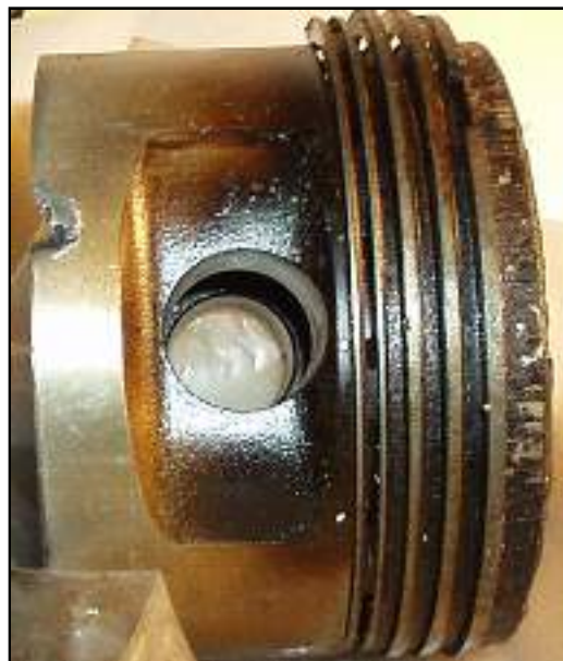
The damaged piston found at engine teardown.
