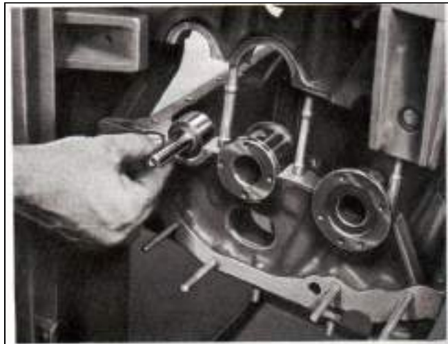
Figure 27. Installing Starter Pinion Pivot
