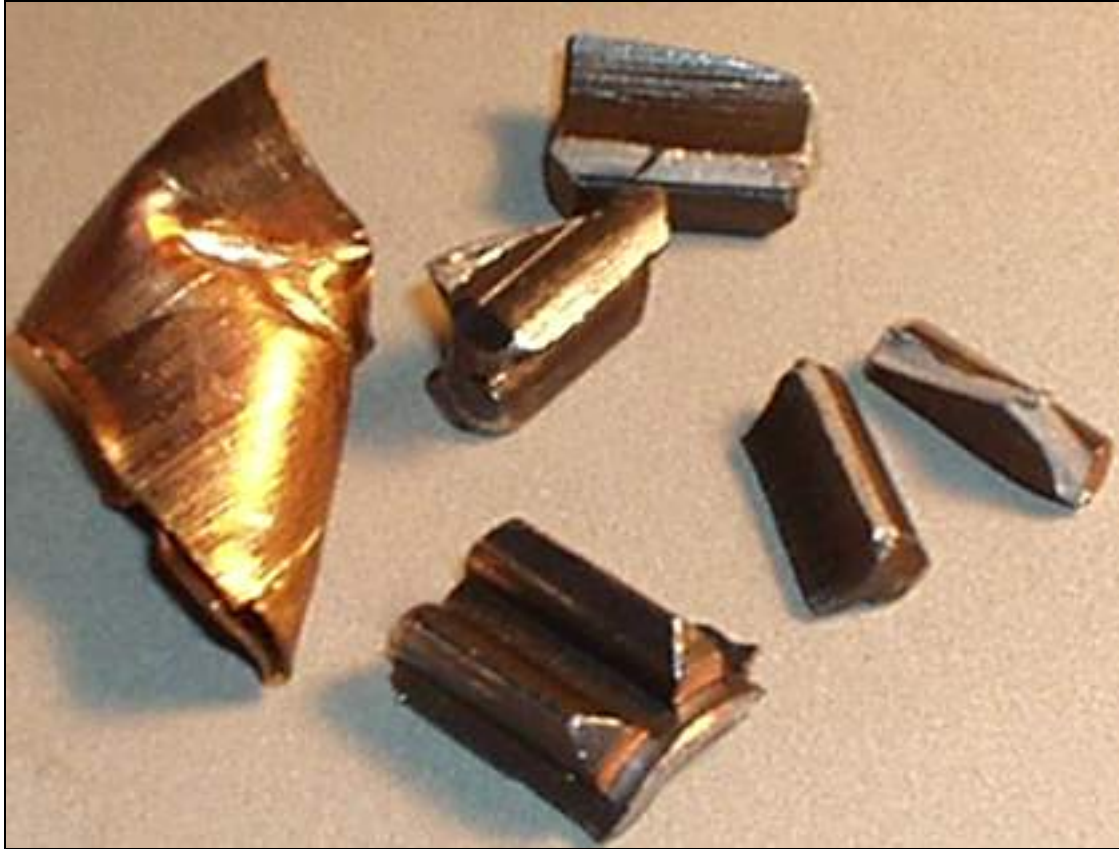
The damaged piston found at engine teardown.
