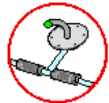
Overwing scupper vent joined to the tank-to-tank vent line
