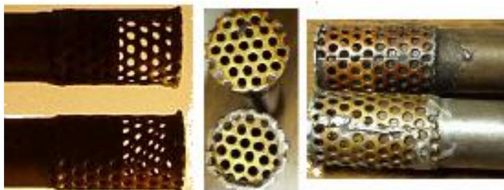
In the middle, the end solder seal, good and poor. The left and right pix show how half of the mesh part is blocked by the tube and solder, with about 5/8ths inch of the mesh open to pass oil when a suction is established by the pump. As John Warren noted, his low oil pressure was at least partially caused by the
