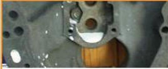
Using milk instead of oil, I filled the oil screen cavity with milk when the accessory case was at about 19 degrees to the tail, much more than the usual 12 degrees of a resting plane. Note the milk in the bottom of the oil pump cavity and the milk that can be seen on the "ledge" which is the highest point of the levelled milk in the oil screen cavity.
