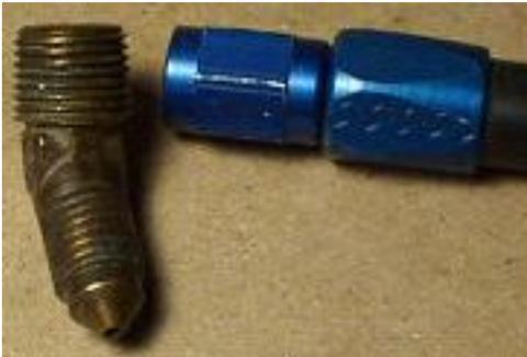
*This is a picture of the oil pressure gauge fitting on most of the engines, size two, though later O-200's used size four fittings and hose. Note the 1/16ths inch hole in the fitting; oil fed in through it would be a slow (the intention of the small hole is reducing oil loss if the line/hose to the gauge breaks) process and getting the fitting out and back in are difficult if one uses that method.*
