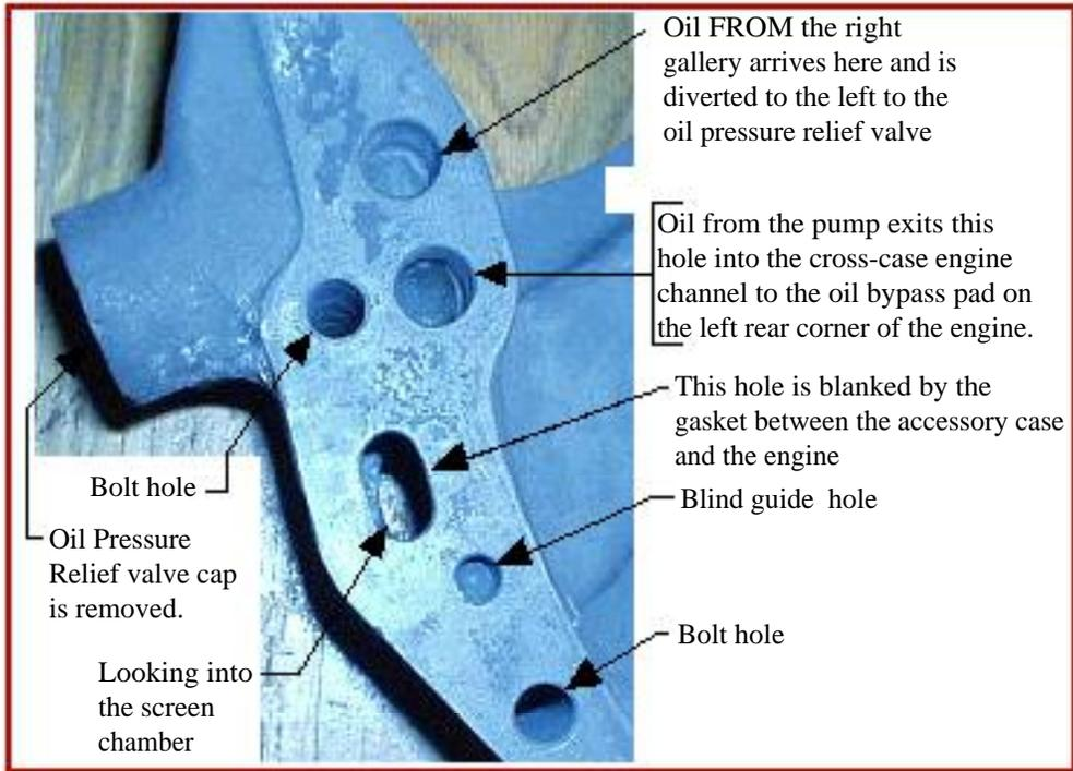
Without an accessory case on one's lap, it is confusing to the extreme to try to follow the pictures from the Continental books and write-ups so this is how the oil is routed on the right side (you are looking at the pump side) of the accessory case.
