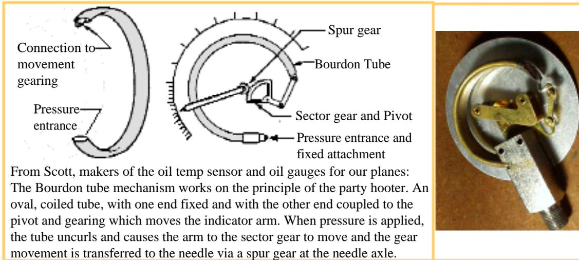
From Scott, makers of the oil temp sensor and oil gauges for our planes:
