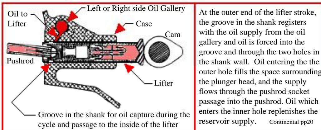
*During loss of pressure, it is true that the lifters' oil reservoir supplies would eventually be depleted and the lifters would be clattering, but by that time the “silent” bearings would have been damaged, along with*
