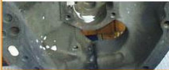
Tilted more than five degrees nose down and still no significant transfer of milk to the oil pump cavity. What does make some move into the oil pump cavity is an extreme right wing high attitude. And sloshing side to side makes some shift as well.
