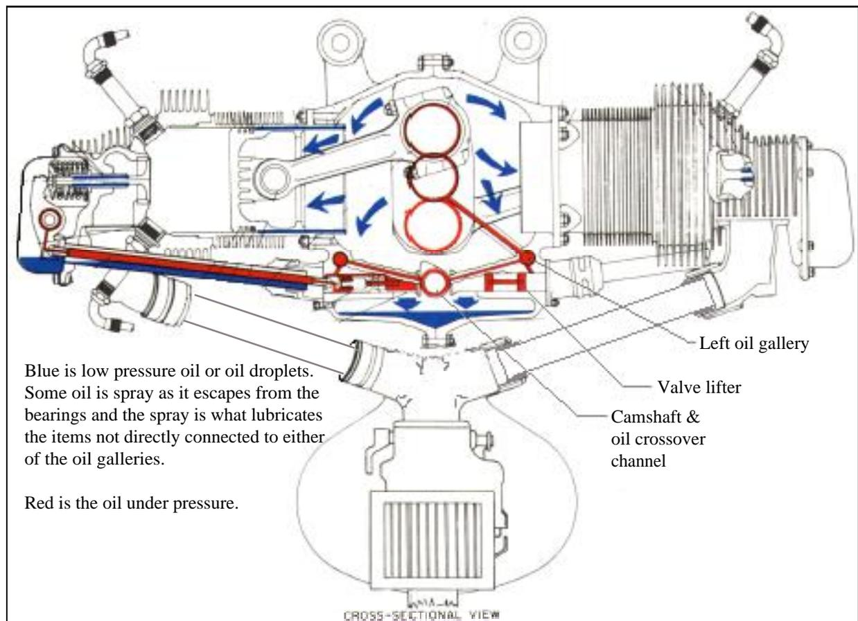
This figure, also from the Continental overhaul manual, but corrected and annotated, serves to show how the oil gets from the left gallery to the right gallery (via a channel cut in the forward bearing portion of the camshaft at the front bearing (but in the shaft, not the bearing) and a bit more of the reservoir and path of
