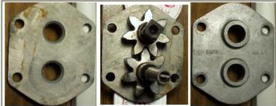
On the left is the inside of the plate. I tried to angle it to show the partial shiny contact marks where the gears seal to the wall, but was not very successful. On some plates, the gouges are such as to be significant and require replacement of the plate, as will wear of the shaft support shoulders. The center figure shows the gears and the plate and the right is the other side of the plate.
