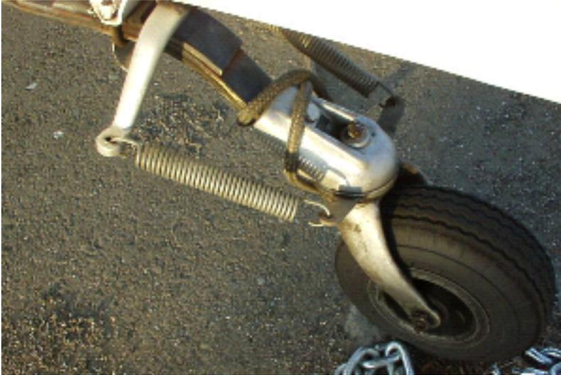
Maule with a Scott 3200 and Maule compressible type steering springs. In this picture, it is easier to see that the two compressing elements pass through the center of the spring at about 90 degrees from each other. Barely perceptible is that the wire of one spring is slightly larger than the other.
