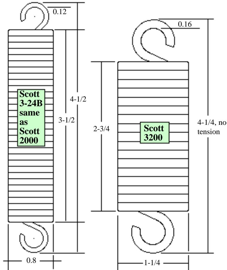
**Steering Spring Sets for the 3200 and 2000 (3-24B) Tailwheels**
