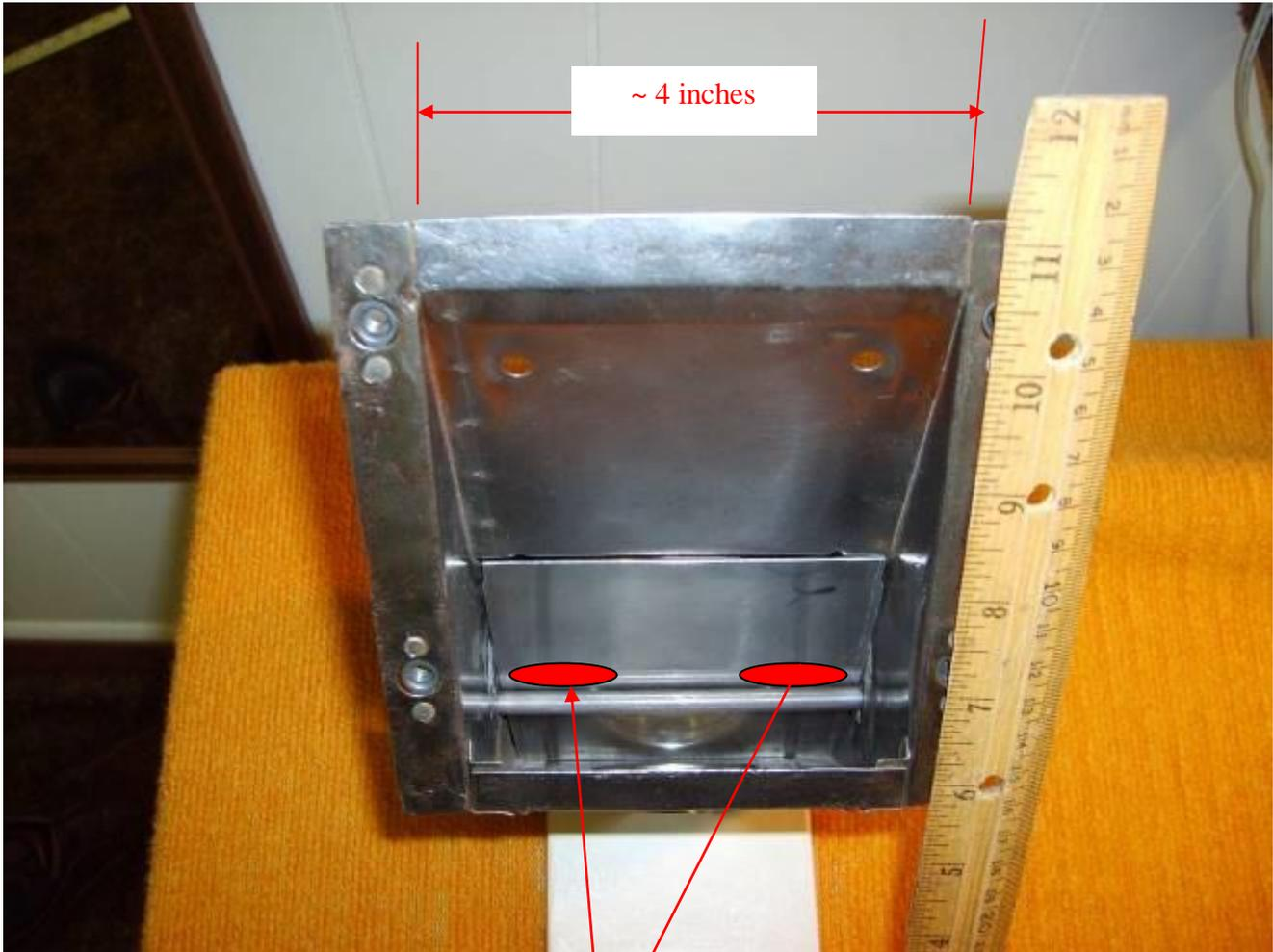
Weld here (Weld #'s 2 and 3). Remove #4-40 screw after each weld, in sequence
