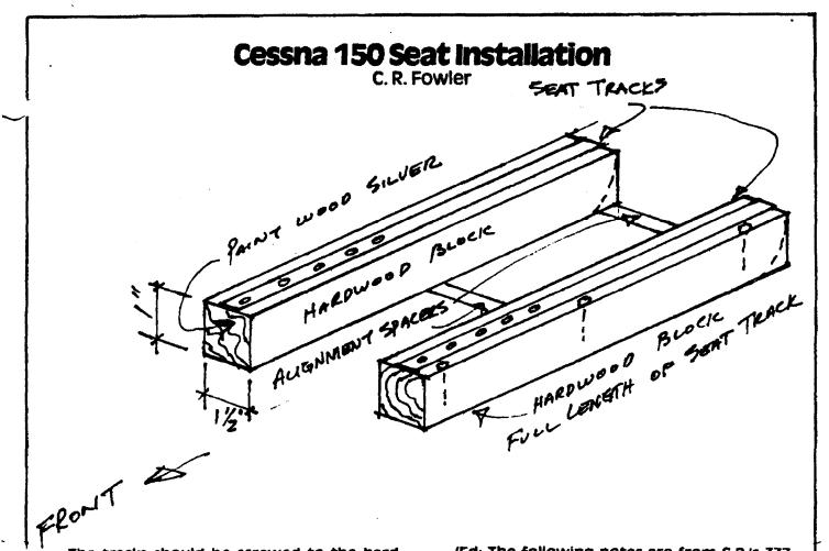
The tracks should be screwed to the hardwood blocks and aligned with the seat before installing. Make a set of spacers so that when you install the tracks they will be lined up properly or you will have a lot of grief.
