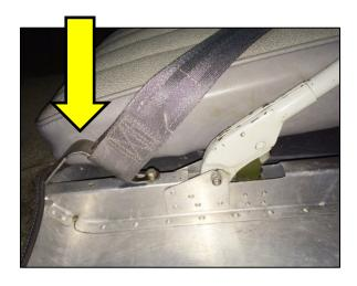
The result of this service bulletin to alert all 120/140 owners to check their seat belt brackets for the most current part, which should be made of steel and not aluminium. Basically, it's pretty easy to determine the composition material of your bracket, all you need is a magnet.
