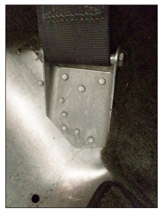
SLN-10 covers this situation as well. Supposedly starting with s/n 8775 at the factory all aircraft subsequent had this mod done right out of production. Oddly enough I've found later s/n aircraft that didn't have the mod, so be vigilant and check this regardless.
