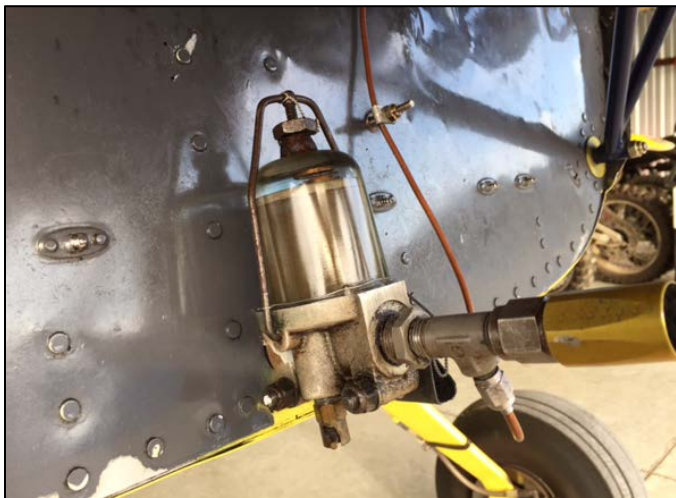
Fuel Strainer as mounted at the bottom of the firewall
