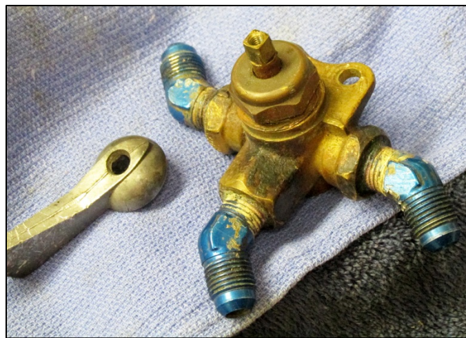
Remove small set screw and pull selector handle off.
