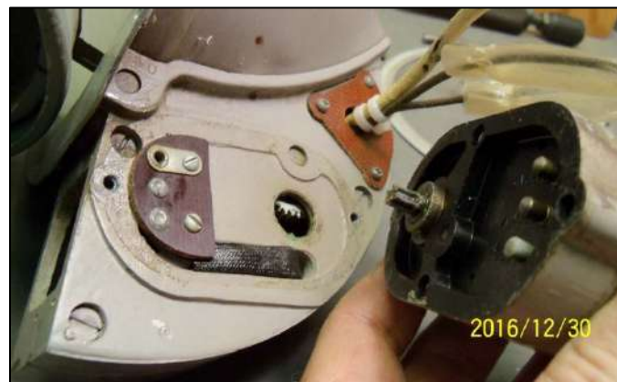
Remove motor to apply grease to gears
