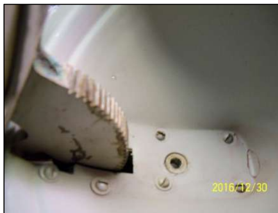
Sector gear exposed with lamp back shell removed.
