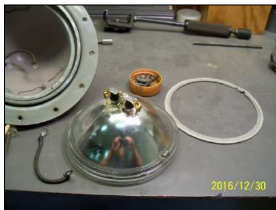
M4522 lamp bulb, retaining snap ring and ground wire, disconnected & removed from back shell.
