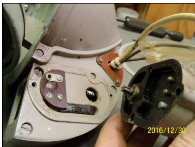
G2905 motor removed, exposing drive and sector drive reduction gears and electrical spring loaded contacts.
