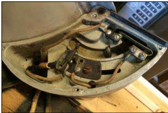
Close-up of sector gear striker contact arm at mid travel with both Up and Down limit switches closed.
