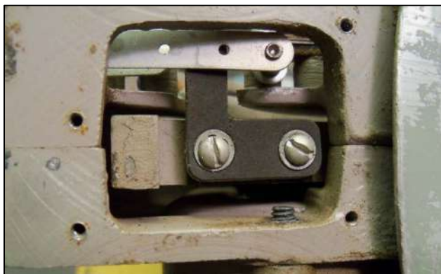
Sector gear striker arm and Up-limit switch close-up.
