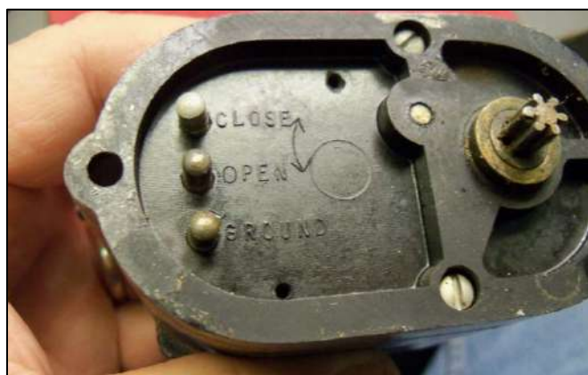
G2905 motor contact markings and drive gear close up.
