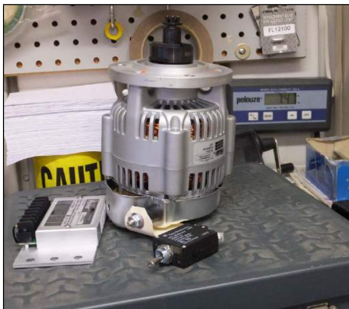
New alternator and voltage regulator on the scale – just under 7 1/2 pounds.
