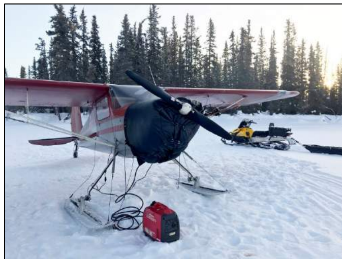
An electric heater can be powered by an external power source.
