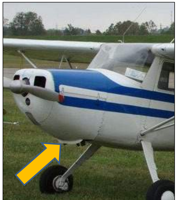
Added cowling lip for increased cooling adds to drag.
