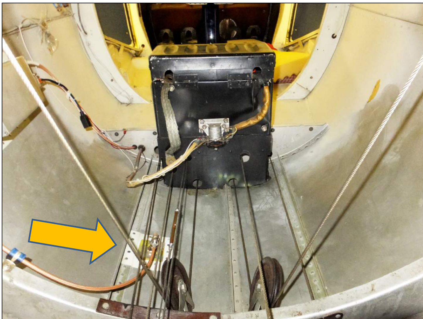
Antenna mounted on the belly of the airplane – everything aft of the battery.
