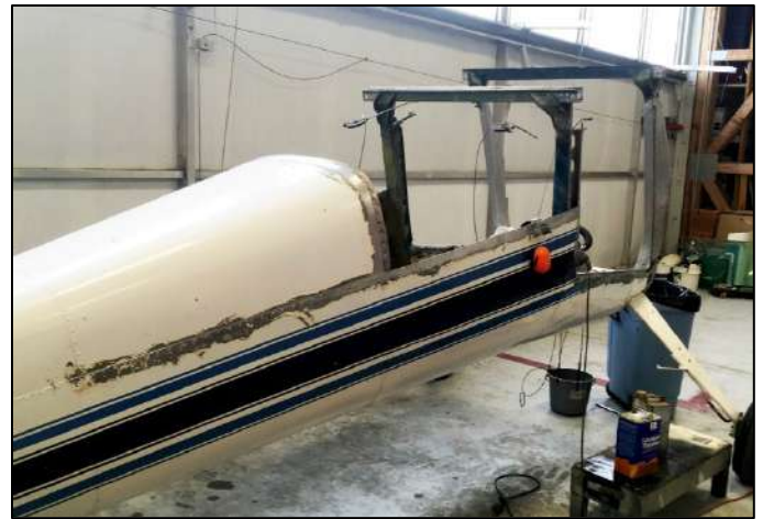
Cabin top off and turtle deck skins removed. Uno still sitting on its own three feet.
