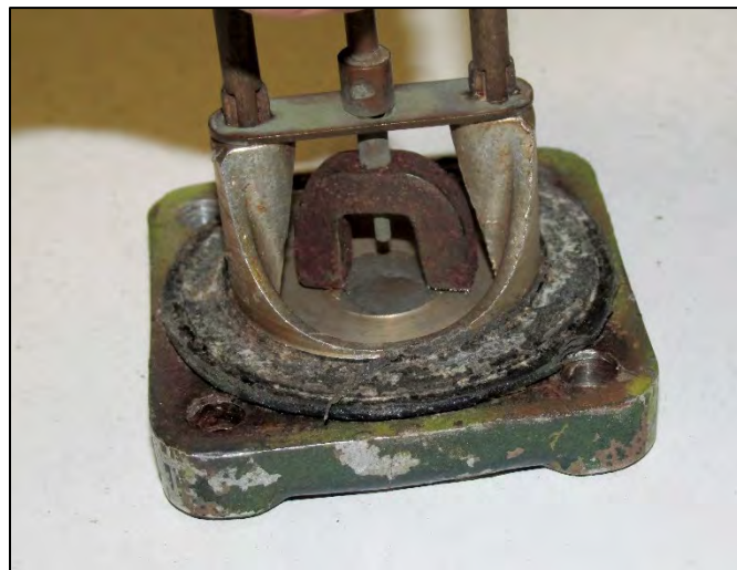
The old seal is often hardened, which is why cranking down on the mounting screws rarely solves a leak.
