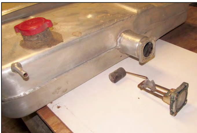
Removing the mounting screws and extracting the fuel gauge from the tank.
