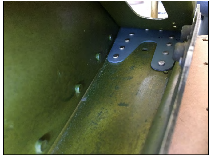
Beautifully installed door post doubler. David Lowe's supplemental type certificate (STC)
