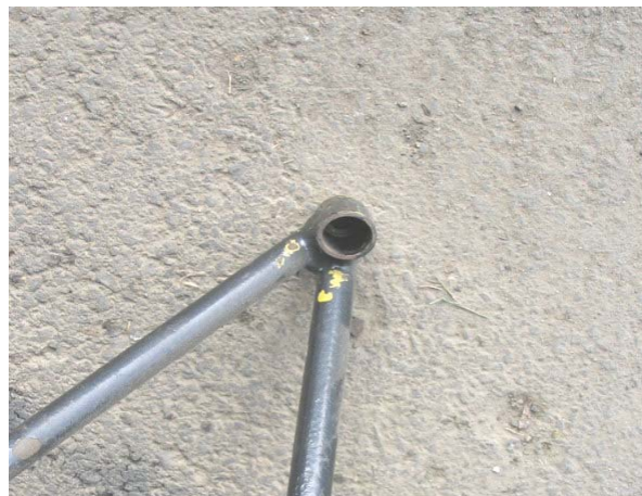
Older Cessna 'hollow tube' C-85 mount
