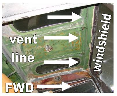
removed the venting tubes, etc. and put on just individual tanks with no venting hook ups.
