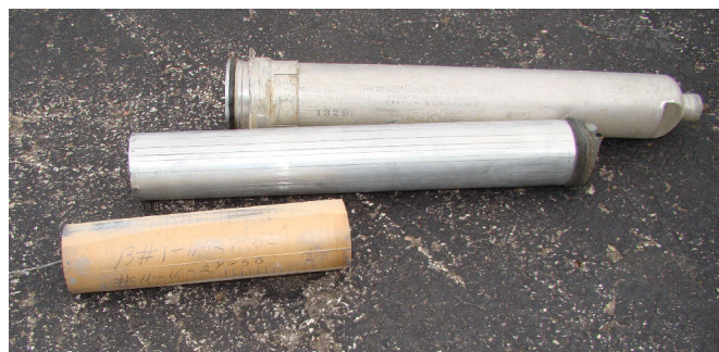
Outside flare housing, inner flare tube and flare cartridge.
