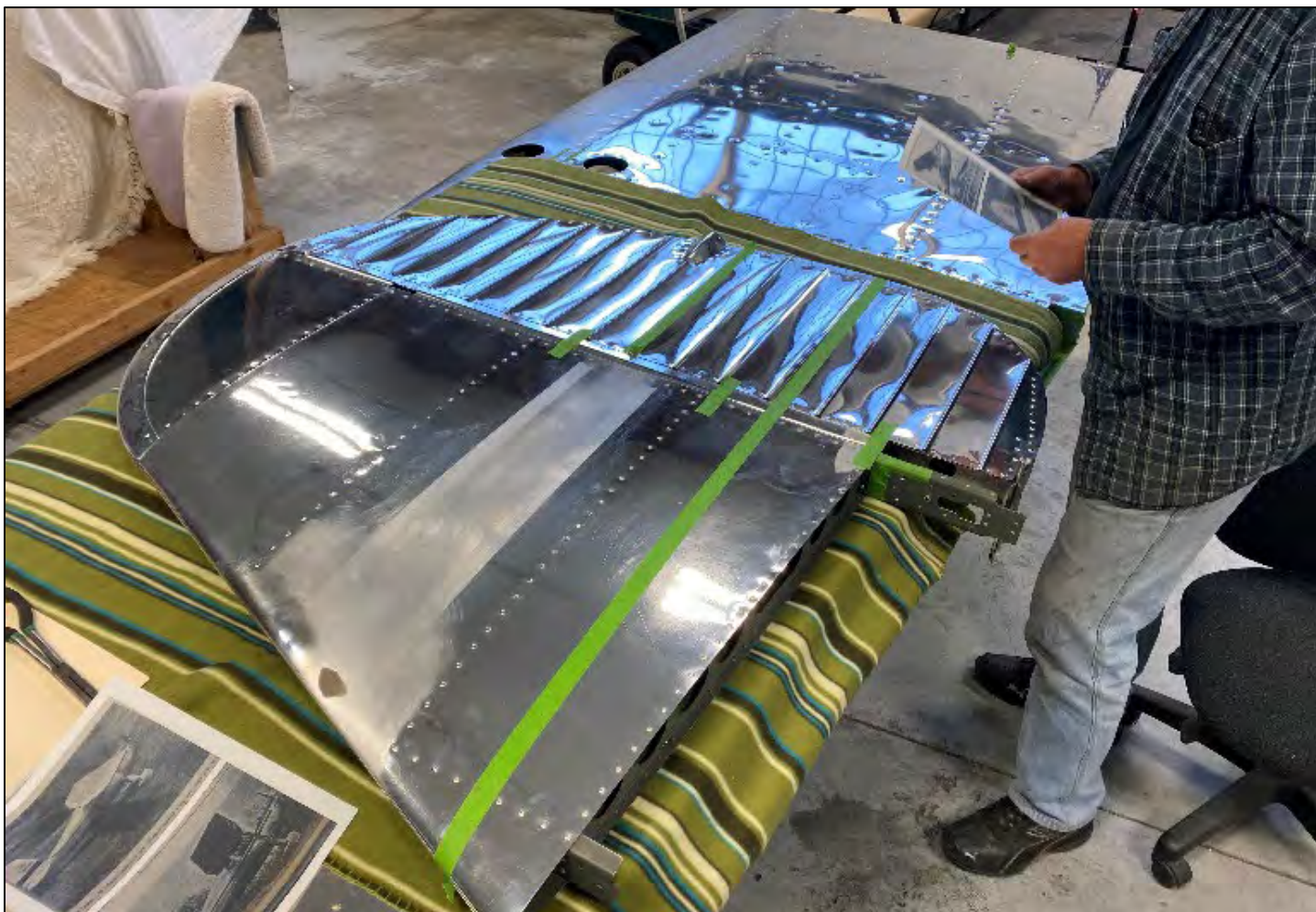
Laying out the stripe in the vertical fin and rudder using old photos to get proper placement
