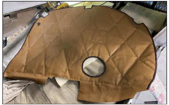
Firewall blanket before and after installation
