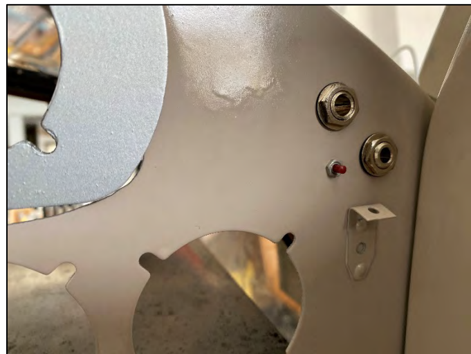
Headset jacks installed in the common location
