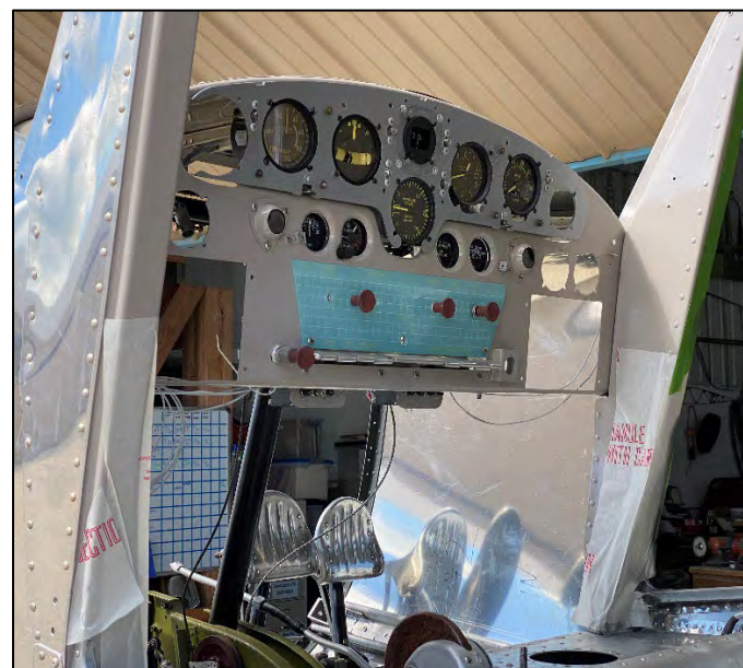
Instruments installed and ready for the radios
