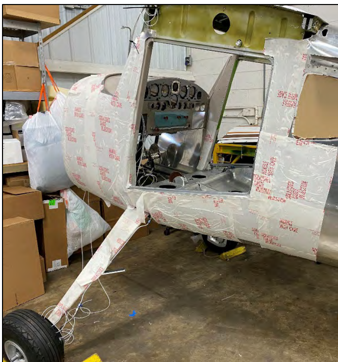
Protective film applied around the cabin prior to radio installation
