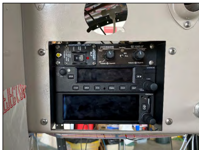
New radios installed in the panel
