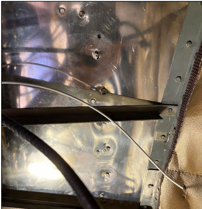
Size #5 rivet tails for the windshield strap
