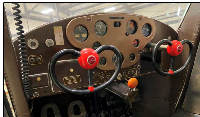
Original 1946 panel where the GE radio was removed and donated to UNO.
