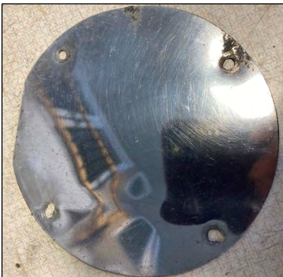
Old stabilizer inspection panel – ugly elongated holes
