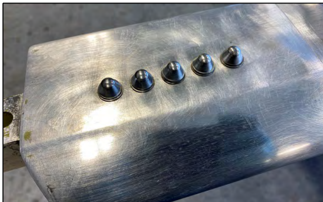
Wing struts cleaned around rivets
