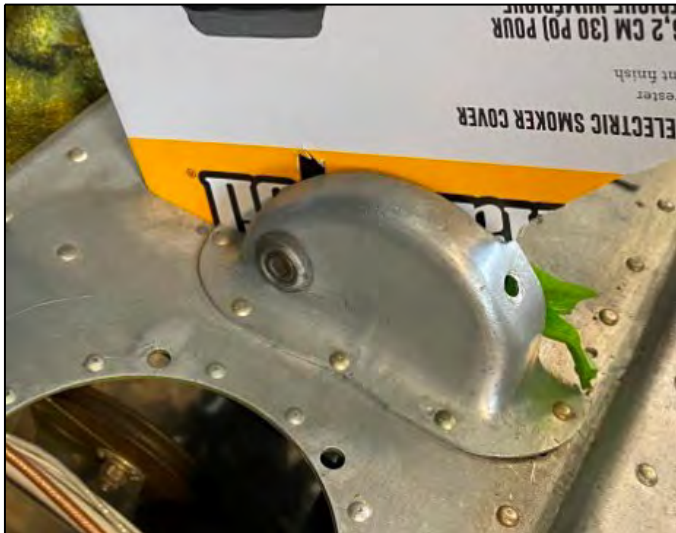
Fabricated barrier to prevent polish compound from contaminating the trim wheel.
