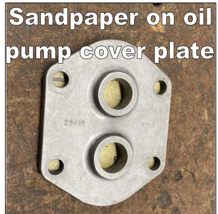
Oil pump cover plate front and rear sides
