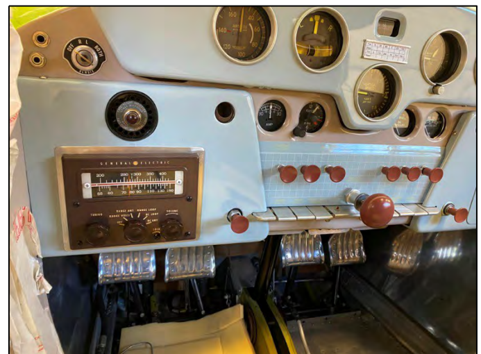
New radio cover with original GE radio installed in UNO's panel.
