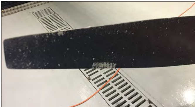
The face of this blade shows excessive wear in the black paint.
