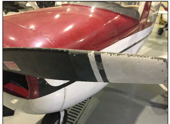
The leading edge of this blade shows no dents, but the paint shows excessive wear and should be addressed.
