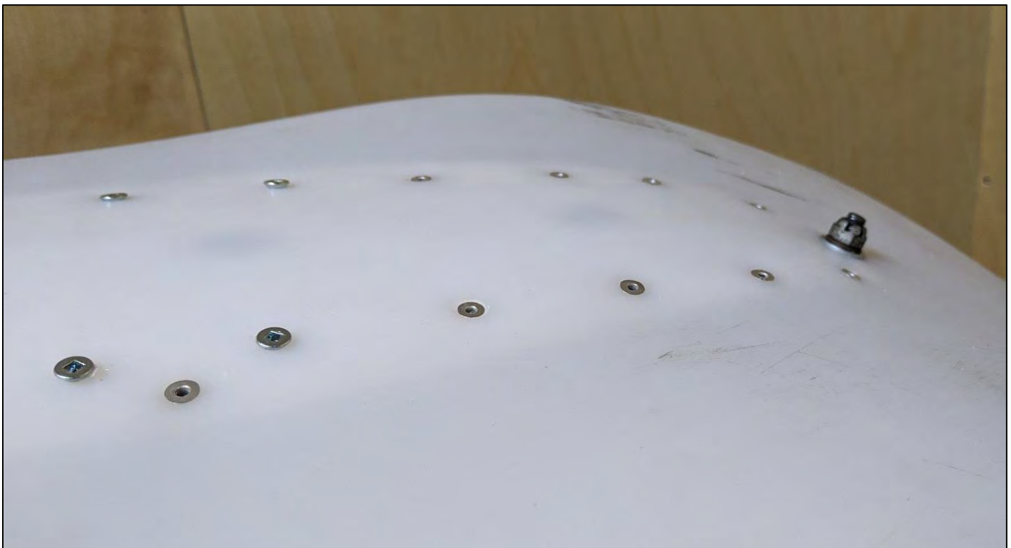
Attaching the UHMW sheet plastic in place prior to cutting and filing to final size.
