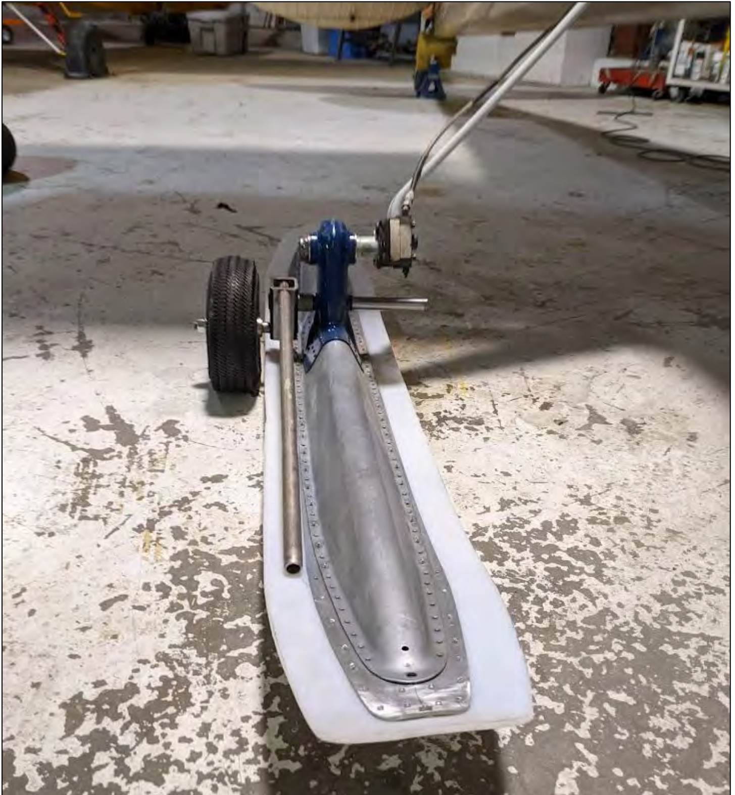
The wheel dollies support the aircraft when the bar is rotated forward, lowering the wheels. Note the extra width provided by the UHMW sheet plastic.
