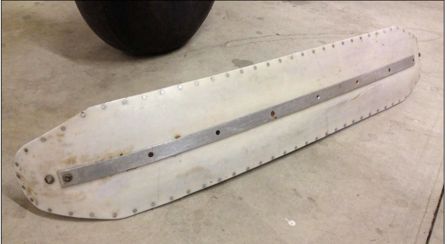
Aluminum Skeg on the bottom of a Federal 2000A
