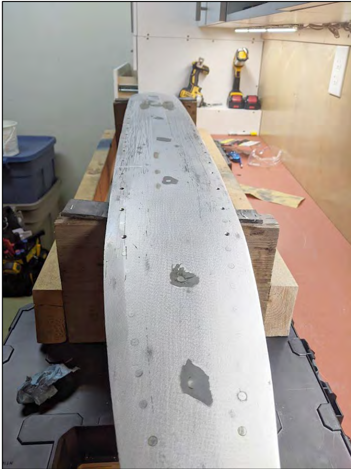
Bare bottoms with the epoxy filler in old skeg holes.
