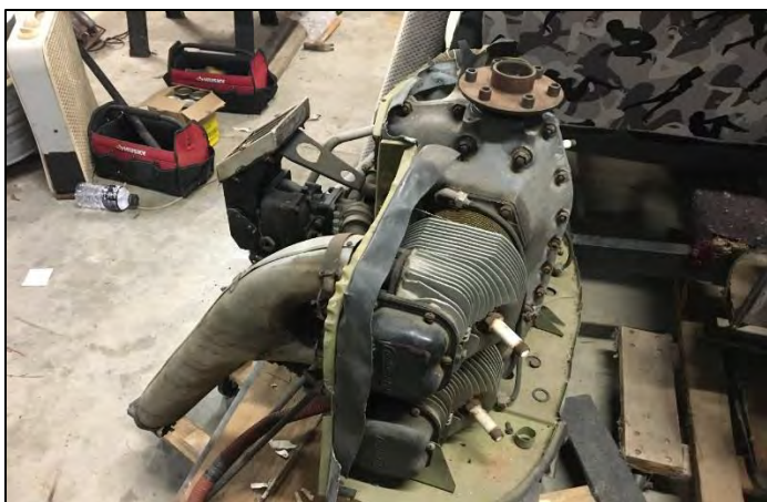
1946 C-85 with accessories, baffling/exhaust.
