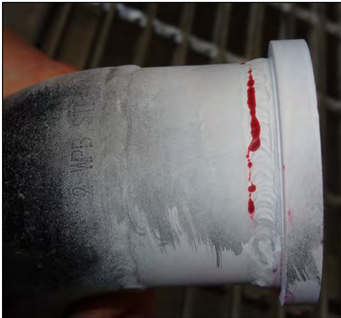
Crack indication using Visible Red Dye and a white developer.
