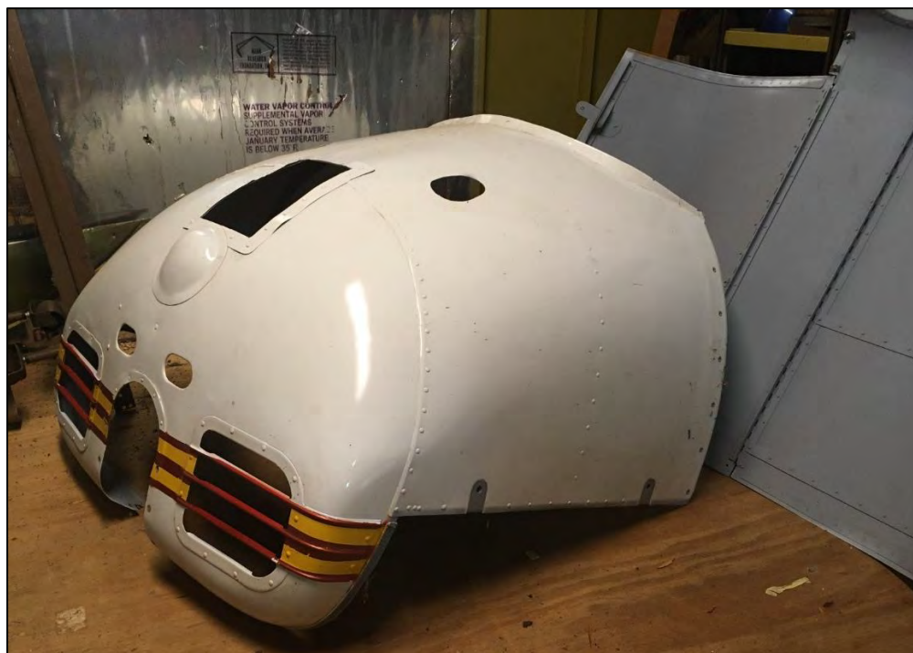
An honorable mention for my dad's inventory, he has a complete cowling that has been extended for the Lycoming O-235 installation.
