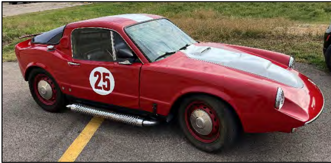
1967 SAAB Sonett, a metal frame, fiberglass body car with a 1500cc V4 engine.
