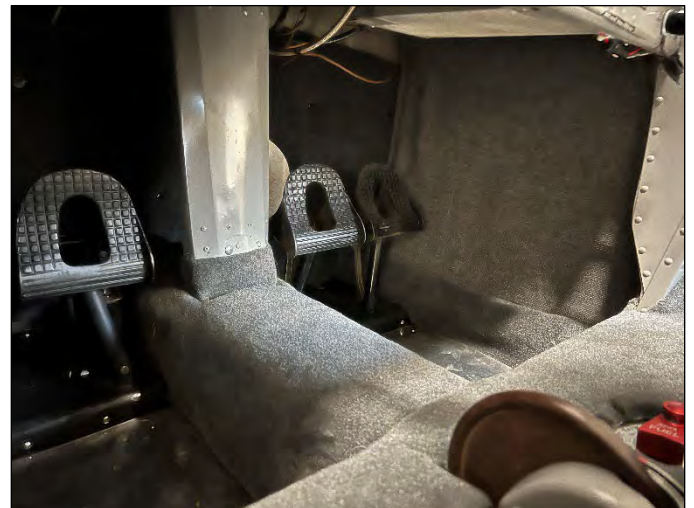
Toe brakes on 1946 Cessna 120/140
