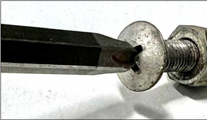
Common Phillips head screwdriver doesn't fit properly in a Reed and Prince screw head
