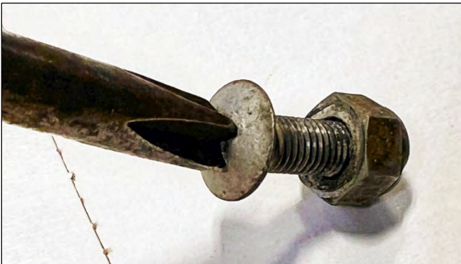
The proper Reed and Prince screwdriver in the same screw
