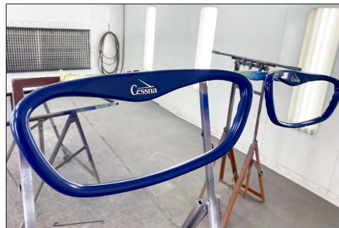
Fixtures used to secure yokes in paint booth
