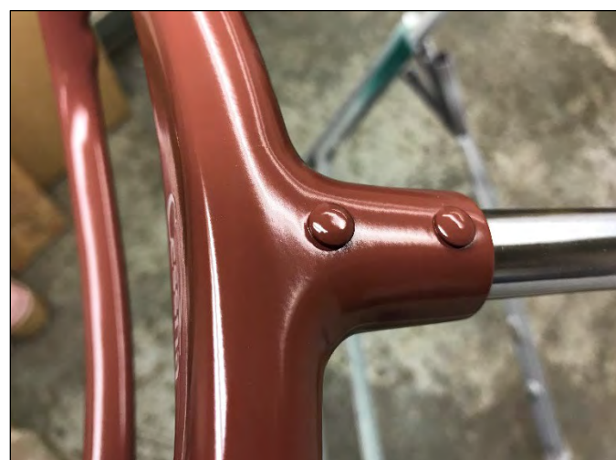
Rivets installed and then painted for longer protection
