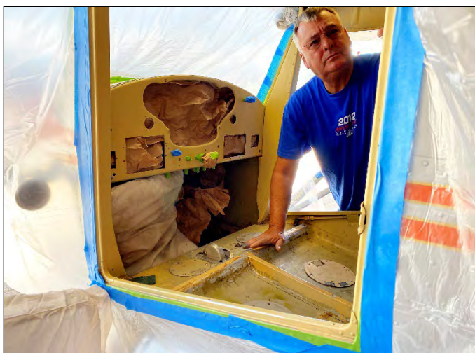
The refresh begins – prepping the original yellow interior for the new paint
