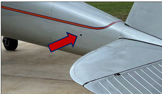
The tail pull handle also eliminates the need to push/lift against the elevator during movement
