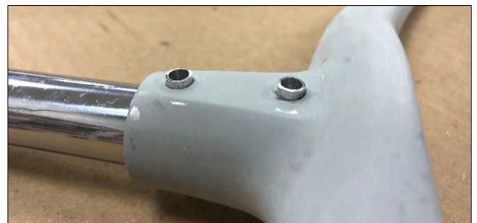
Tubular (hollow) rivets secure the yoke to the shaft
