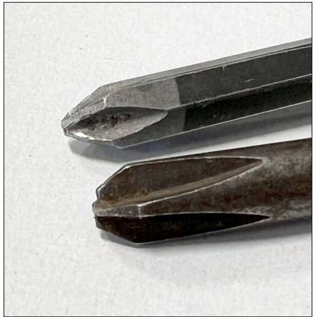
Common Phillips head screwdriver on top Reed and Prince screwdriver on bottom
