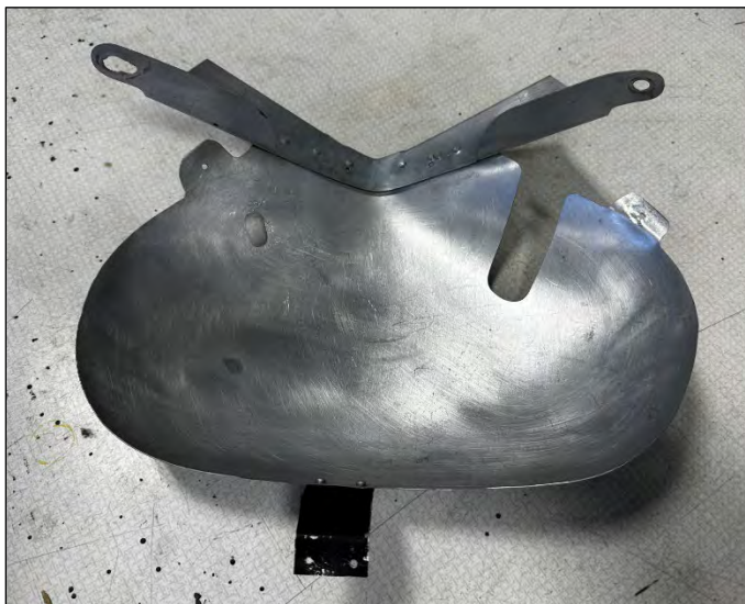
Oil tank cooling baffle (not common)
