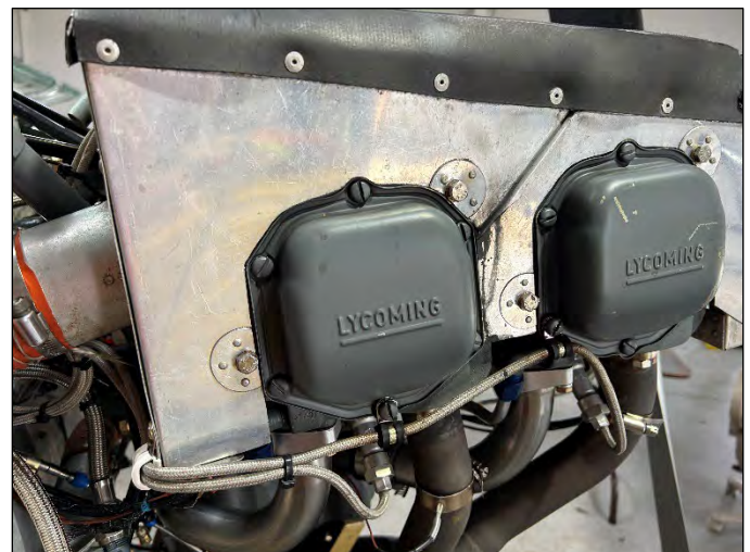
Nice tight fit around the cylinder heads forces the cooling air down through the cooling fins of the heads
