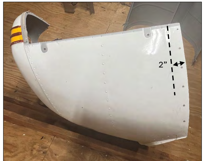
The overall length was increased due to the specific engine mount that was chosen for this aircraft
