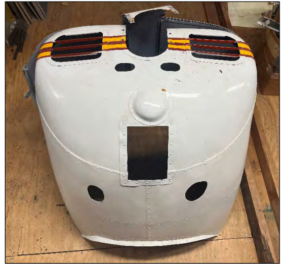
Notice the bump on the nose bowl to provide clearance for the starter
