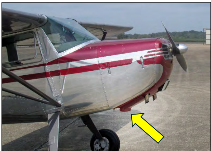
Continental O-200 installation with an additional cooling lip to aid airflow
